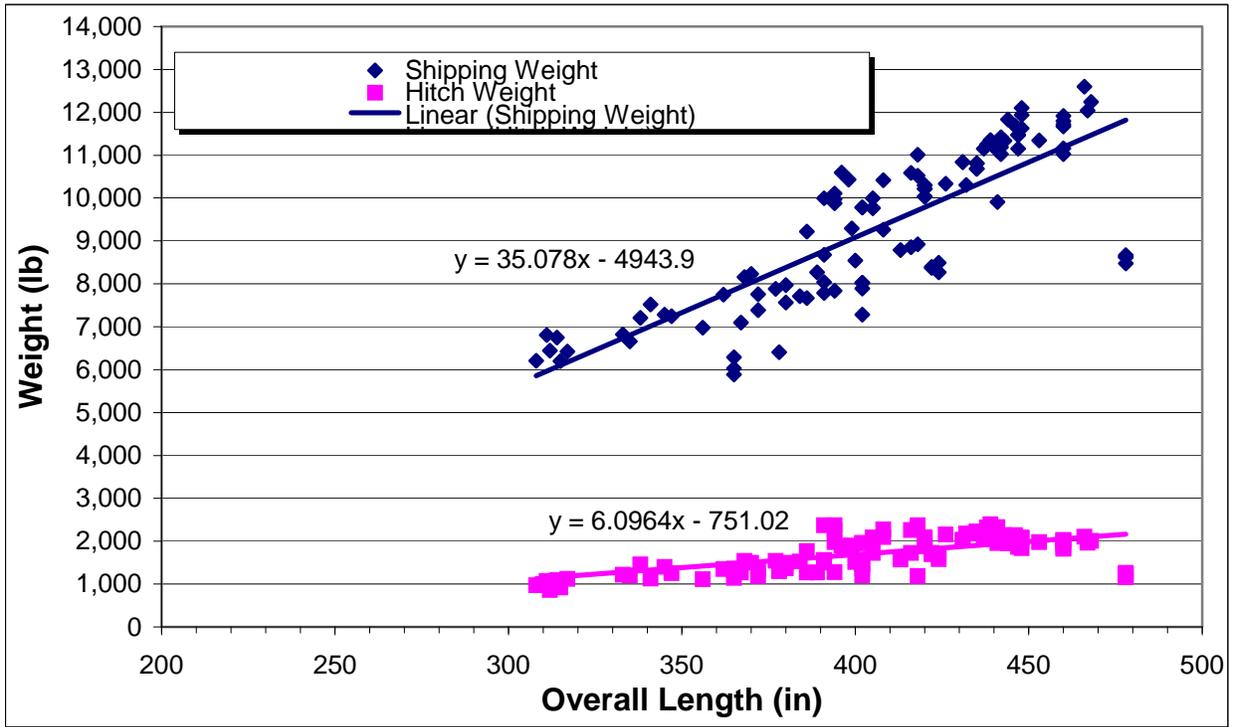
Figure 7: Weight and Hitch Load for Travel Trailers
